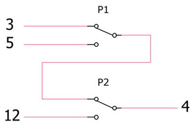
Example of Fan Motor and Spark Transformer connection
